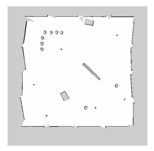
Unknown areas (gray) should be removed and treated as free space. Create a logical matrix based on a threshold. Depnding on your image, this value could be different. Occupied space should be set as 1 (white in image).
