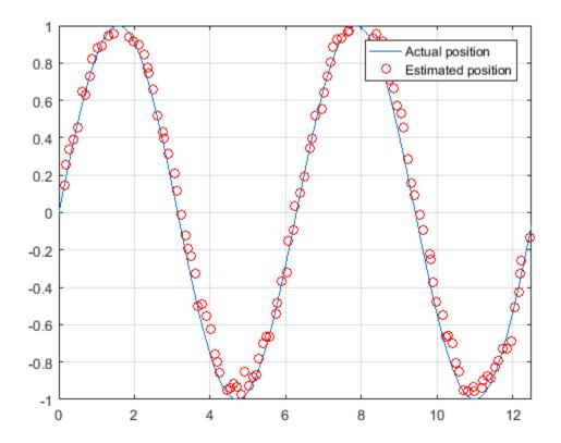
The figure shows how close the estimate state matches the actual position of the robot. Try tuning the number of particles or specifying a different initial position and covariance to see how it affects tracking over time.
